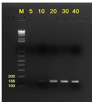
Figure 5. Electrophoregram of amplification of the N fragment of the rabies virus gene at different primer concentrations (5, 10, 20, 30, 40 pM) Note: M – DNA marker; lanes 1-5 correspond to the specified concentrations Source: developed by the authors
